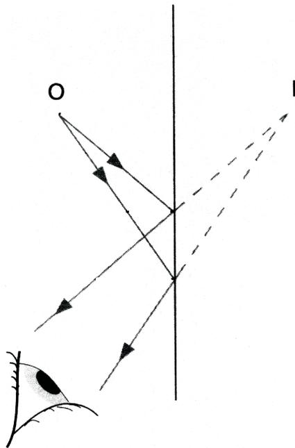
Figure 1. A typical textbook diagram showing how reflection in a plane mirror produces a virtual image (I) of the object (O). The dotted lines indicate virtual rays. (After Duncan and Kennet, 2001).
